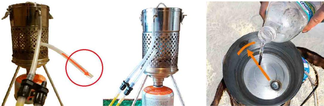
7. If the water does not circulates even when water boils, disconnect the heater from the stove and cool water down enough or disconnect the water coming out (below) hose from the boiler, discharge whole air and reconnect it. At this time, flame should be reduced to the smallest.
