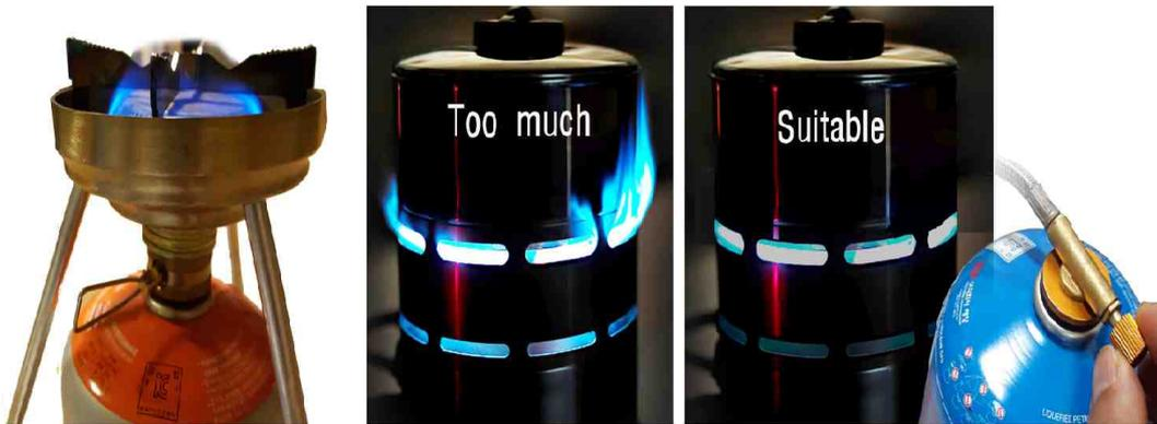
9. Adjust the flame size properly with the fuel supply adjusting valve.
