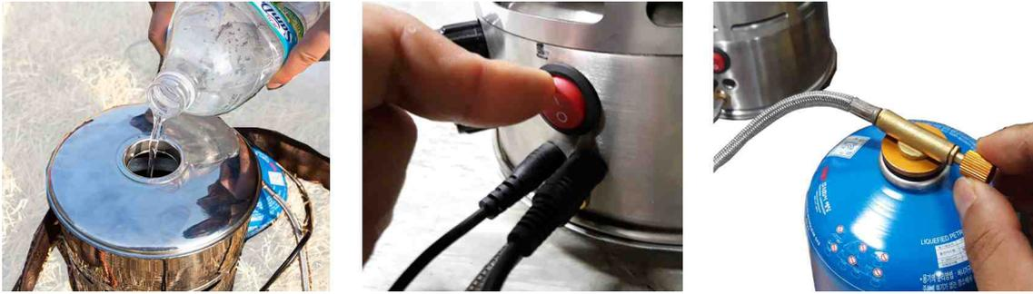
5. Open the water tank lid, fill it with water, and lock the lid. (Minimal/Single pad 900ml, Double/Triple 1,000ml)
